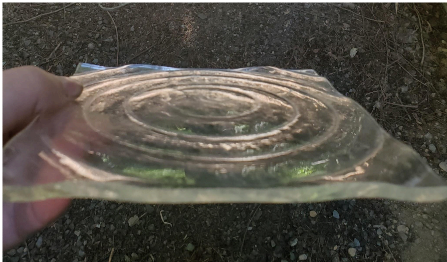
Sample pieces created using a ring mold for slumping.
