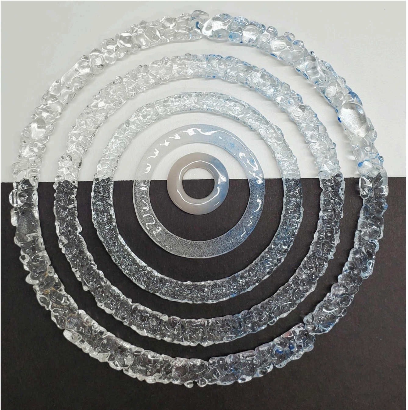
Sample Contour Fuse rings made with different sizes of glass frit.
