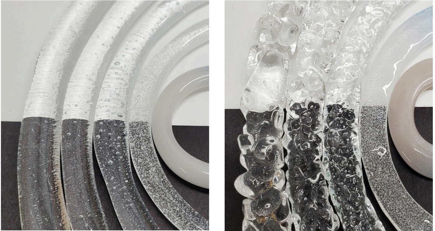
Side by side comparison of Full Fuse Schedule (left) and Contour Fuse Schedule (right) rings showing bubble size and distribution.
