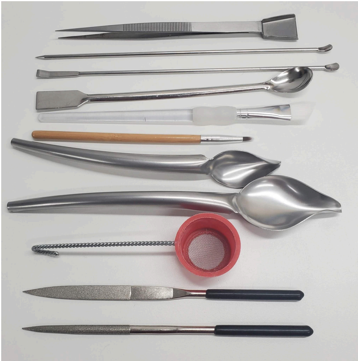
Just a few of the many useful tools in manipulating frit for filling the mold
