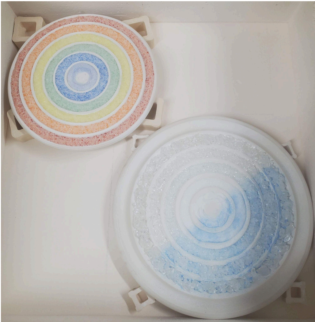
Filled molds loaded and ready for firing. Note the kiln posts raising the molds off the surface of the kiln shelf.
