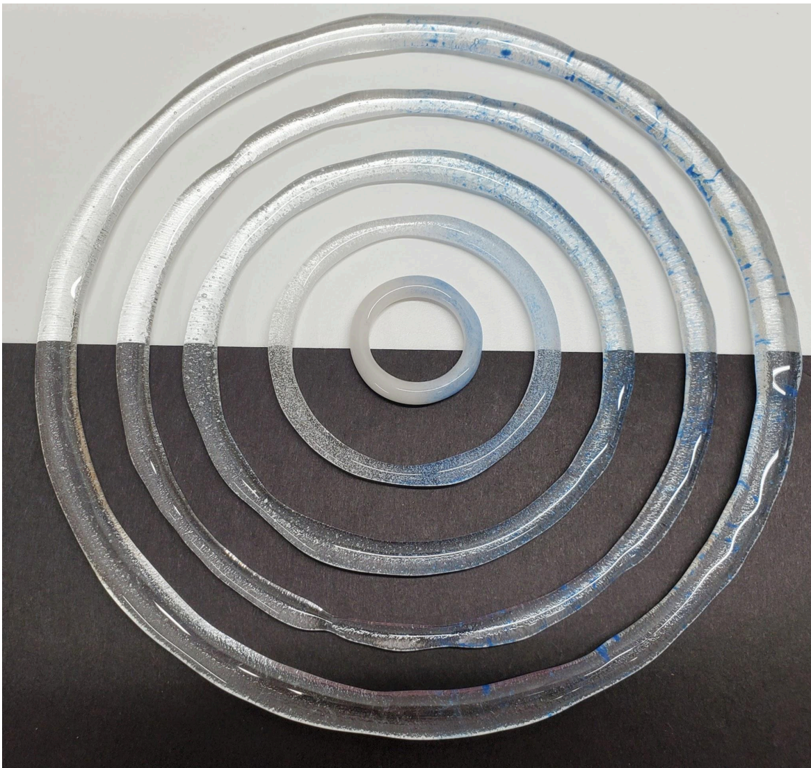
Sample Full Fuse rings made with different sizes of glass frit.
